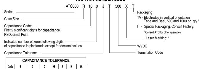
The above part number refers to a 800 R Series (case size R) 10 pF capacitor, J tolerance (±5%), 500 WVDC, with T termination (Tin Plated over Nickel Barrier, RoHS Compliant), laser marked, and tape and reel packaging.
